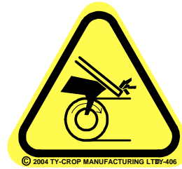
TY-406: Crush hazard—avoid rotating conveyor belt
