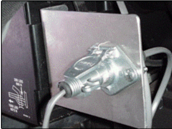
Figure 16: Electrical connection on tow vehicle
