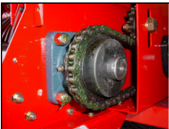
Figure 25: Grease fitting on base model (one at left rear, one at right rear)
