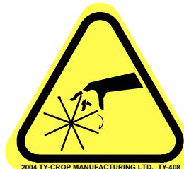
TY-408: Shear hazard—avoid rotating spinner disks
