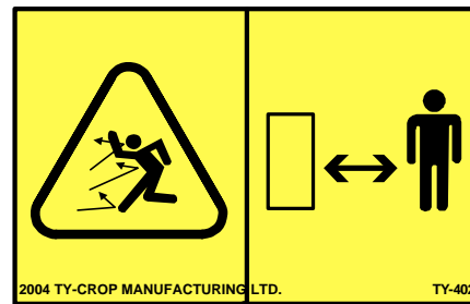
TY-402: Projectile hazard—stay a safe distance from the machine
