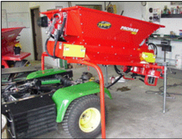
Figure 14: Installing the ProPass onto the tow vehicle (or uninstalling it onto the storage stand)
