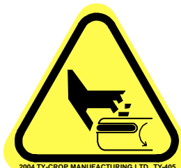
TY-405: Shear hazard—avoid rotating shaft
