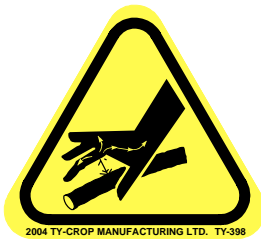
TY-398: High-pressure fluid hazard—avoid high-pressure hydraulic lines
